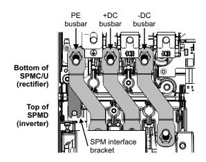
Docking kits are available that provide the necessary hardware to directly mount the SPMC to an SPMD.
